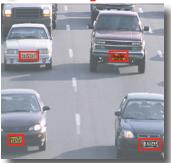
iQ-LPR is a highly accurate multi-lingual License Plate Recognition system which can detect and automatically read the required characters in any images. The system will recognize the presence of a vehicle when it approaches (without any external trigger) to read the plate and compare it against multiple databases.
